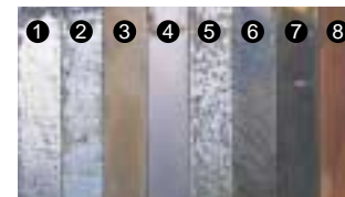
Test result using non-genuine brake fluid
