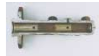
Test result using non-genuine brake fluid
